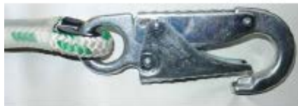
Gate Stuck Open
