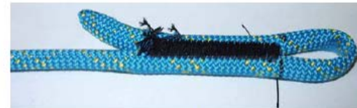
Eye Splice Broke / Loose Stitching
