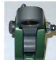
Missing Split Ring
