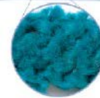
Abraded / Frayed Rope (Excessive Wear)
