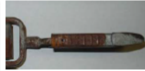
Rusted / Excessively Corroded Hardware
