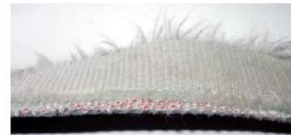
Red Warning Center Exposed (Webbing)
