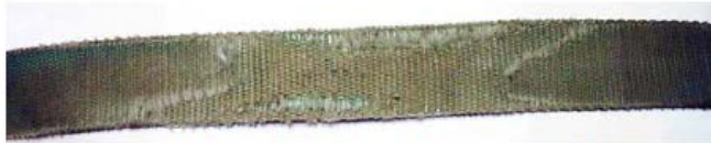
Abraded / Frayed Webbing (Excessive Wear)
