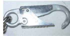
Distorted / Bent Hardware
