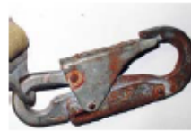
Rusted / Excessively Corroded Hardware
